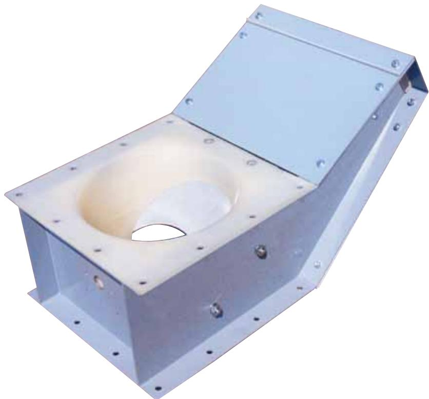
The VDI Inclined Slide Valve is innovative as a whole. Its inclined blade forms an eye-shaped aperture with the asymmetrically tapered inner body. The wider the eye is opened, the more material flows through, the further it is closed, the more the material flow is reduced.
