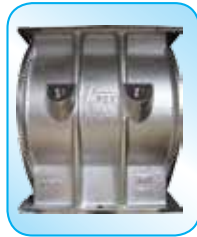
Lateral air venting bores as standard Used for: - extracting excess air from rotor pockets - decreasing air pressure inside the casing - increasing throughput
