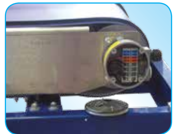
8 Electric motor drum
